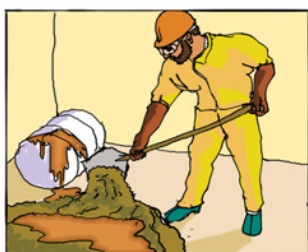
Surround the spill
