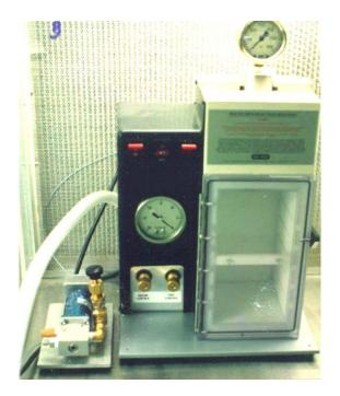
Fig 1: Micro projectile bombardment facility (BIORAD)
